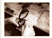
Rebecca Minkoff and Shane Baum created over 12 combinations of custom made plastics that are unique to the collection. These combinations are applied to a flat piece of zyl [acetate] that is manufactured in Northern Italy. During the cutting process a computer controlled router cuts the acetate directly from an AutoCAD® drawing.
